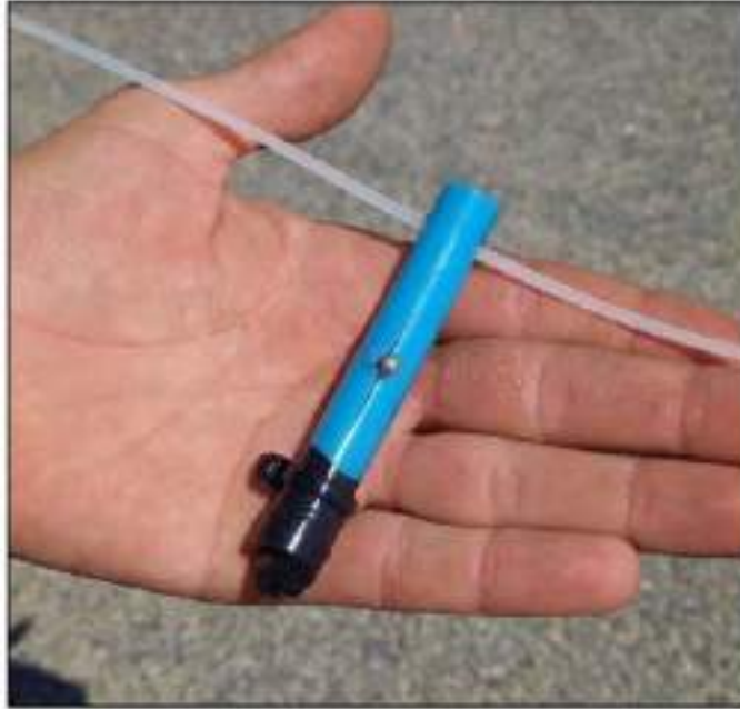
Figure 5.2.4.5-3: View of Acoustic Transmitter Installed Horizontally in a Plastic Protective Tube for Range Testing Exercises
