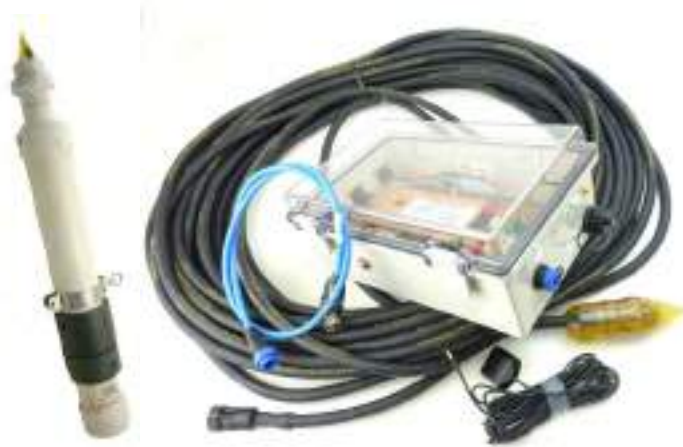
Figure 5.2.4.5-1: ATS Hydrophones (SR3001 on left and SR3017 on right) Proposed for Evaluation during Phase I
