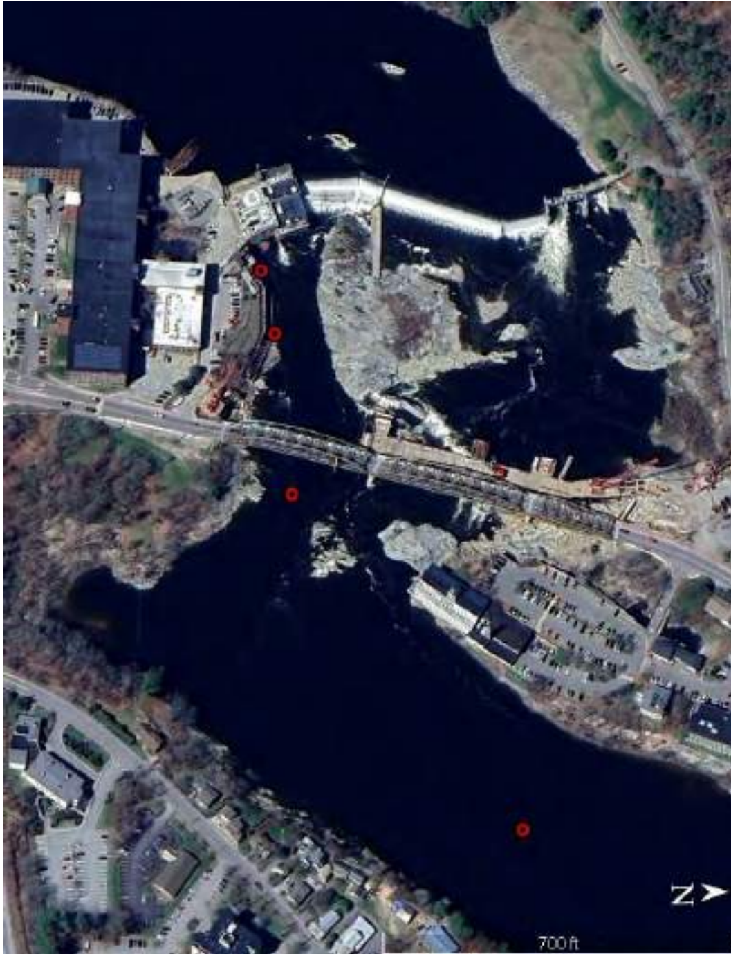
Figure 5.2.4.5-2: Proposed Hydrophone Locations for Evaluation of Detection Range and Efficiency during Phase I Study
